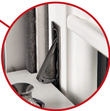
Spring-loaded restrictor shown limiting how far the window can be opened. Press and slide window to open position.
